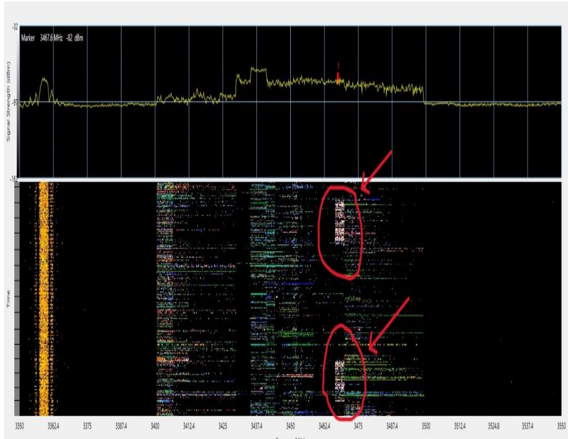
Figure 1(a): Shows external Interference within a 5G signal in the 3500MHz band.
